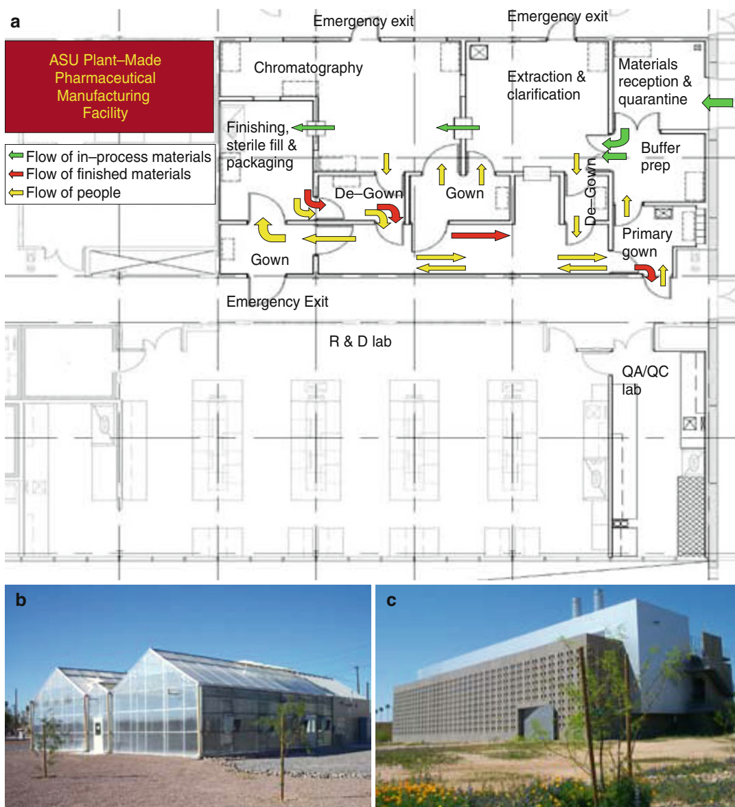
Fig. 8.2 cGMP production facilities for NVCP VLP vaccine. (a) The design of the central bioprocessing suite. The arrows indicate the unidirectional flow of in-process materials (green), purified final product (red), and people (yellow). (b) The BSL-2 greenhouse facility for plant biomass generation and NVCP expression. (c) The Plant
