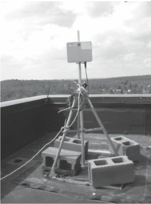
Figure 3-1. Rotorod (rotating air impactor) air sampler. (Courtesy Rose Vrtis, University of Wisconsin – Madison.)
