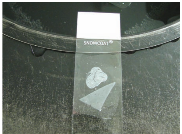
Figure 4.43 The same tissue sections have now been floated onto a glass slide ready for staining
