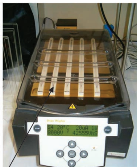
IEF 'coffin' tank holding an immobilized ampholyte strip.
