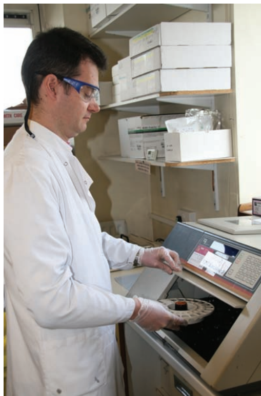
Figure 6.14 Antibiotic assays being performed on a TDX analyser
