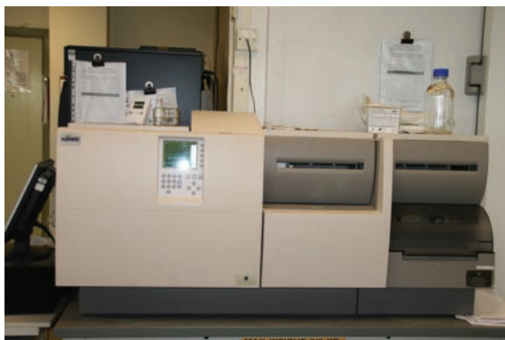
Figure 6.12 Vitek system for bacterial identification and sensitivity
