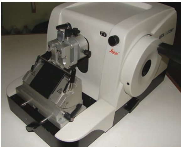
Figure 4.41 An example of the type of rotary microtome commonly in use
