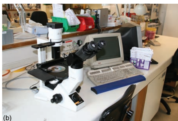
Figure 6.7 (a) Fuchs–Rosenthal counting chamber and (b) inverted microscope for urine microscopy
