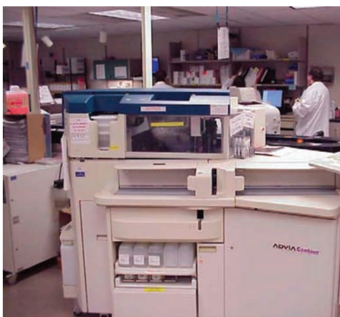
Figure 5.2 Example of an autoanalyser in a clinical chemistry laboratory and a bench top sample dilution and distributor system
