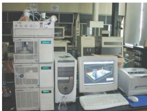
Figure 5.19 Illustration of HPLC equipment and the core component — the HPLC column
