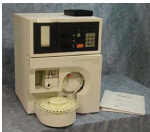
Figure 5.4 Example of a simple flame photometer
