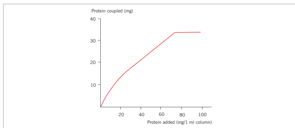
Fig. 60. Ligand coupling to HiTrap NHS-activated HP.
