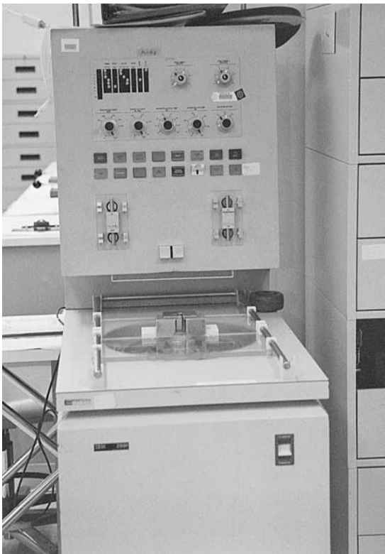
Figure 11–3. Automated cell washers such as this may be used to prepare washed RBCs or to deglycerolize frozen RBCs. (Courtesy National Institutes of Health, Bethesda, MD.)
